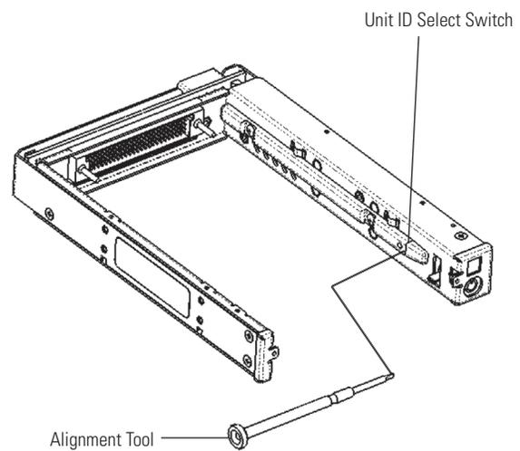
Figure 3: Unit ID Select Switch Location
