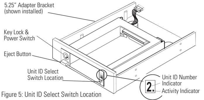
Figure 5: Unit ID Select Switch Location
