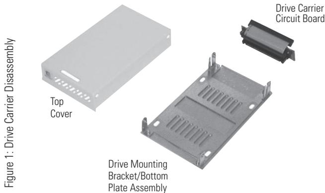
1. Loosen and remove the four (4) M3 Phillips Flat Hd. screws located on the sides of the drive carrier unit. Save these screws for Step 6.
