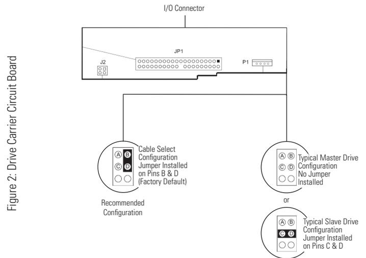
Figure 2: Drive Carrier Circuit Board
