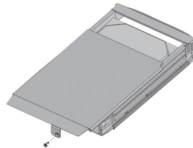
Figure 1: Removing the Cover
