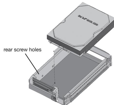
Figure 2: Installing the drive
