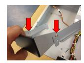
g. To install the USB Type B connector into the rear of the RAX unit, position one screw in the opening on the rear of the RAX unit into the long screw slot, shown in the photo on the right.
