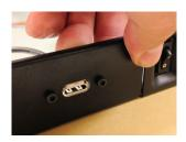
a. Remove the four screws that secure the bay mounting bracket assembly to the RAX unit.
