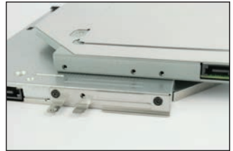
Figure 3. The bracket is attached to the optical drive. Attach it to the rear of the DP27 on top.
