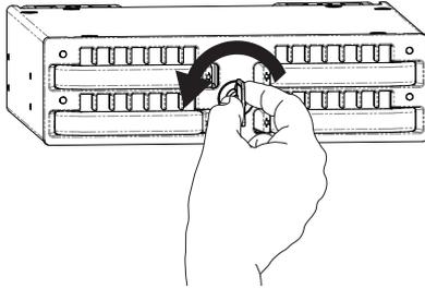
3. Pull the eject tab to the center of the QX448 to open the module cover. Then move the module cover out of the way.
