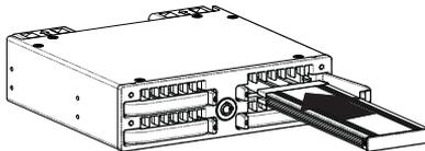
4. Close the module cover until it snaps into place. The SHIPS module will automatically power on when the computer is turned on.
