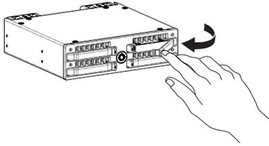
5. You may optionally lock all receiving slots at once by inserting the provided key and rotating it 90 degrees clockwise.
