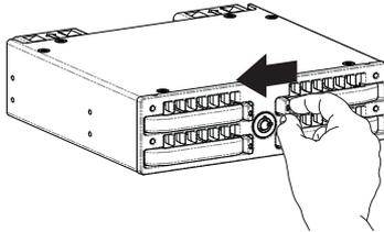
3. Orient a Q80 SHIPS module so that its pins are downward and facing the QX448. Insert it into an open slot on the QX448 receiving frame.
