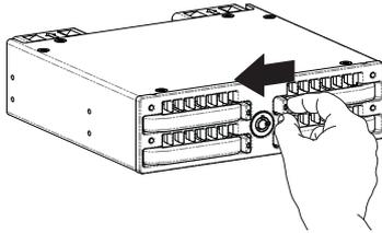
4. Pull the module out of the receiving frame.
