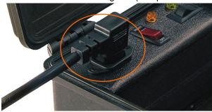
**C.** Plug the other end of the input line cord into the new power source that you want to switch to (such as a portable UPS). The HotPlug power switch will light up, indicating that HotPlug is receiving power. Make sure that a second receptacle on the same circuit is available on the new power source (i.e. a duplex outlet).
