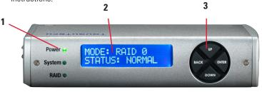
1. Unit Power, System, RAID LEDs
