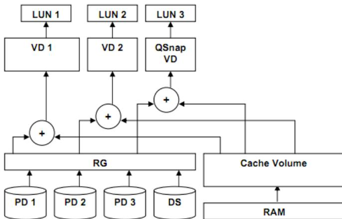
Each RAID Group can be divided into several Virtual Disks. The Virtual Disks in one RAID Group share the same RAID level, but may have different volume capacity. All Virtual Disks share the Cache Volume to execute a data transfers. A Logical Unit Number (LUN) is a unique identifier that the computer uses to distinguish and access SCSI devices.
