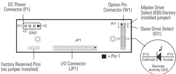
Figure 1: Receiving Frame Motherboard (Rear View)
