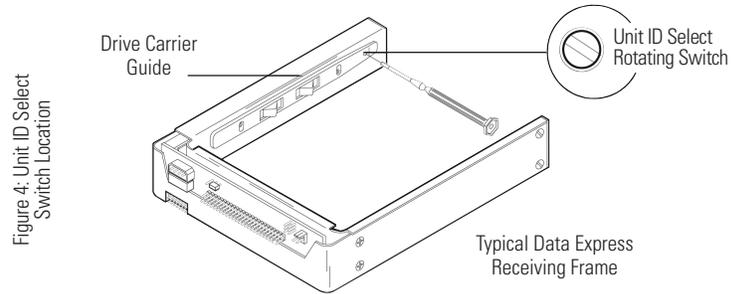
**NOTE:** The lock on the Data Express receiving frame functions as a lock and a DC power switch for the carrier unit. The lock MUST be engaged (turned counterclockwise) in order to supply power to the carrier and installed drive unit.
