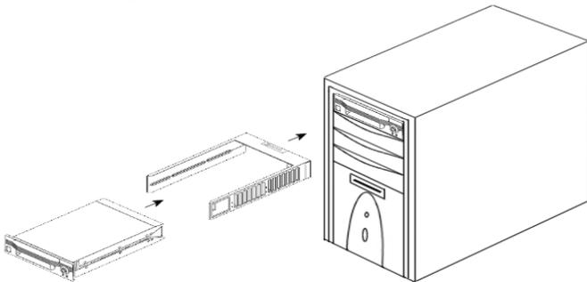
2. Locate an available 5.25" drive bay with external access. Remove the cover of the computer. Identify the 5.25" half-height bay in which the DataPort frame assembly will be mounted. Examine the bay to determine the location of mounting holes or whether mounting rails are required. Remove any filler plates that may be present on the computer.
